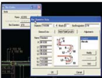
Reinforcing in plan and section is automatically drawn to code.
